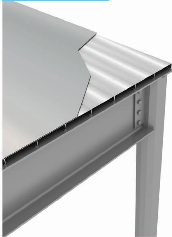
ENTIRE SUB-DECK INSTALLATION
